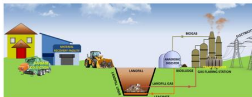
Fig: Consolidated municipal solid waste landfilling system and utilization of leachate and landfill gas for energy generation (Nanda and Berruti 2021).
